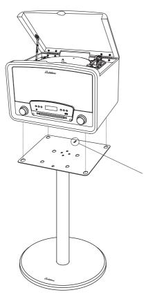
When lowering the RR75 onto stand, place the feet into the holes to ensure stability.
